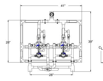
**+NOTE:** The valve will maintain temperature with 0.5GPM flow from the domestic hot water loop when properly installed near the hot water source with a continuously operating recirculation pump.
